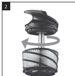
**2 Assemble the squeezing screw,** turning the upper part clockwise until a click is heard.
