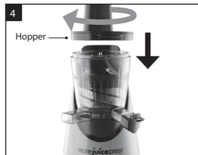
**4 Place the hopper on the drum** turning it clockwise.
